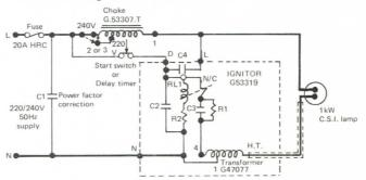
C1 - 175 uF 250 V A.C.  $C2/C3 - 0.22 \text{ \muF } 1000 \text{V}$  $C4 - 0.005 \text{ \muF } 250 \text{V A.C.}$  R1 − 4.7k.∩10W
